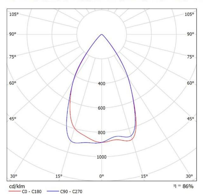
Luminaire: Ledil CN12605\_LENINA-W-DL\_(Bridgelux\_BXRA\_ES\_Rectangle) Lamps: 1 x Bridgelux\_BXRA\_ES\_Rectangle\_(BXRAES-W0802)\_186.209Im@250mA\_P=2.6918W\_I=0.25A
