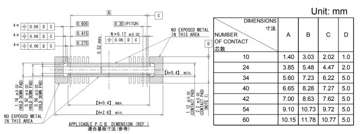
Note 1) Dimension 2.8  $\pm$  0.05 is recommended in case repair is needed.
