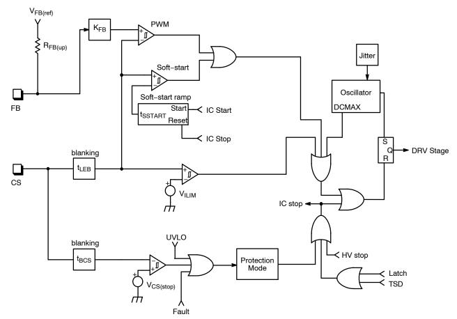
Figure 36. Current Sense Block Schematic
