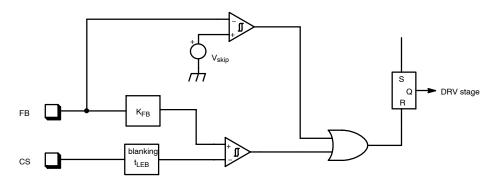
Figure 48. Skip Cycle Schematic
