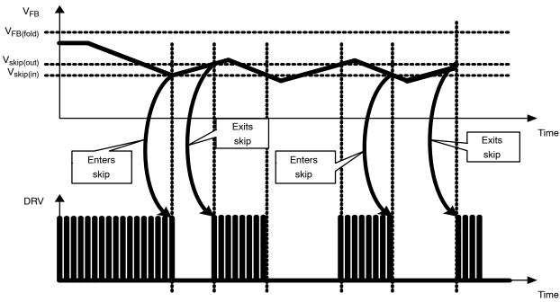
Figure 49. Skip Cycle Timing Diagram
