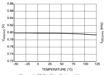
Figure 19. FB Pin Skip-Out Level V<sub>skip(out)</sub>
