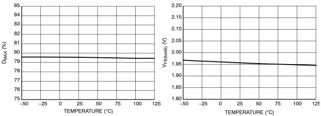
Figure 15. Maximum Duty Cycle  $D_{MAX}$
