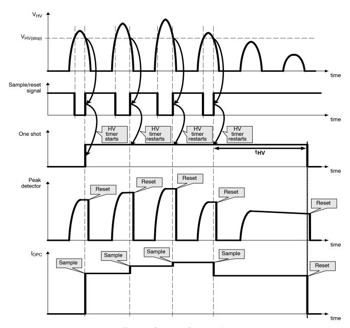
Figure 41. Overpower Compensation
