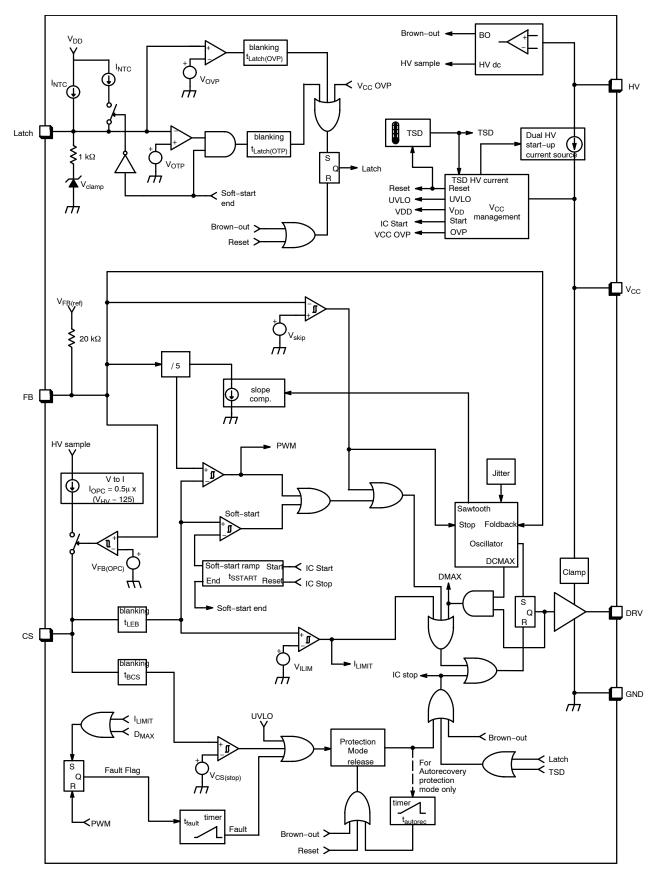
Figure 2. Simplified Internal Block Schematic
