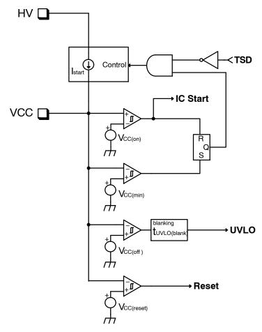
Figure 30. HV Start-up Current Source Functional Schematic
