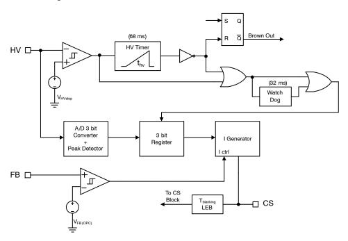
Figure 39. Schematic Overpower Compensation Circuit
