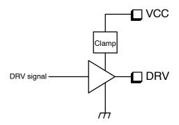
Figure 35. Clamped Driver
