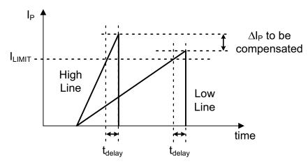
Figure 38. Line Compensation for True Overpower Protection
