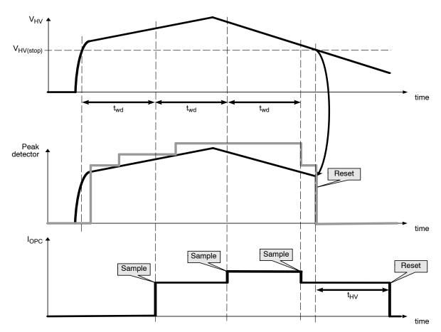
Figure 42. Overpower Compensation
