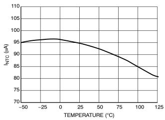
Figure 28. Current  $I_{\mbox{\scriptsize NTC}}$  Sourced from the Latch Pin, Allowing Direct NTC Connection
