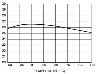
Figure 20. Minimum Switching Frequency f<sub>OSC(min)</sub>
