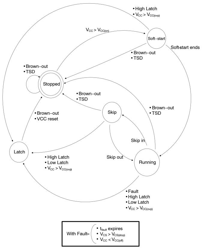
Figure 53. Controller Operation State Diagram (Latched Protection)
