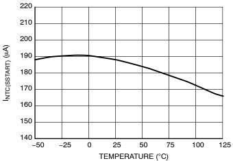
Figure 29. Current I<sub>NTC(SSTART)</sub> Sourced from the Latch Pin, During Soft-Start
