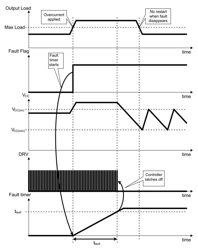
Figure 46. Latched Timer-Based Overcurrent Protection
