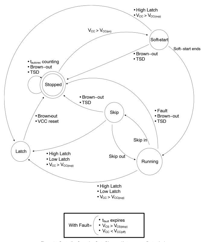
Figure 54. Controller Operation State Diagram (Autorecovery Protection)
