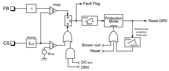
Figure 44. Timer-Based Overcurrent Protection
