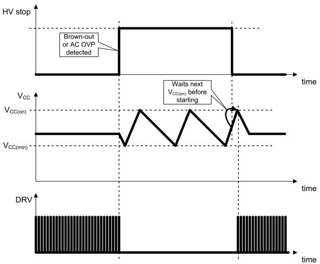
Figure 32. Brown-out Timing Diagram
