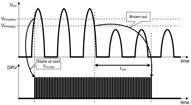
Figure 33. AC Input Brown-out Timing Diagram
