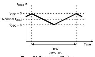
Figure 34. Frequency Jittering
