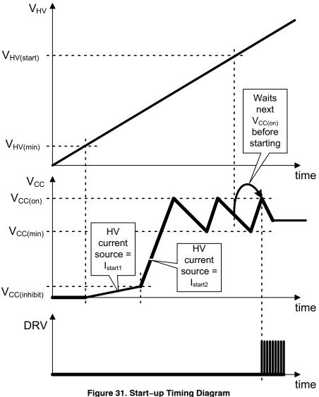
For safety reasons, the start-up current is lowered when  $V_{CC}$  is below  $V_{CC(inhibit)}$ , to reduce the power dissipation in case the  $V_{CC}$  pin is shorted to GND (in case of  $V_{CC}$  capacitor failure, or external pull-down on V<sub>CC</sub> to disable the controller).
