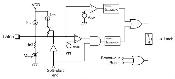
Figure 50. Latch Detection Schematic
