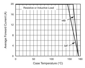
Fig. 1 - Forward Current Derating Curve
