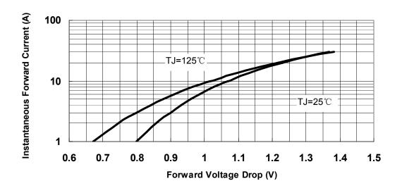
Fig.3-Typical Instantaneous Forward Voltage Characteristics
