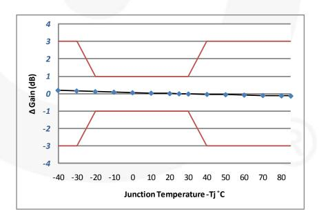
Figure 7. Δ Gain vs. Temperature (Nominal Temperature= 25°C)
