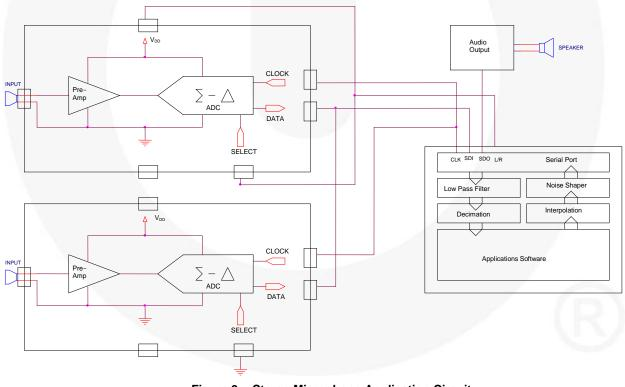
Figure 9. Stereo Microphone Application Circuit
