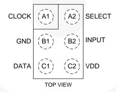
Figure 2. Pin Assignments
