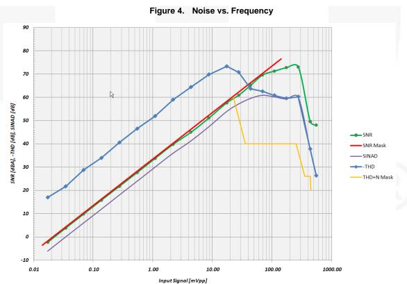
Figure 5. THD, SINDA, and SNR vs. Input Amplitude
