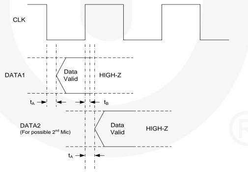
t<sub>A</sub> – Microphone delay from clock edge to data assertion.
