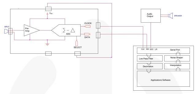
Figure 8. Mono Microphone Application Circuit
