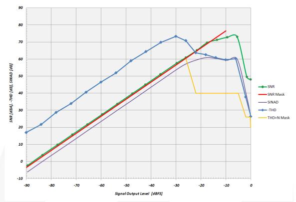
Figure 6. THD, SINAD, and SNR vs. Output Level
