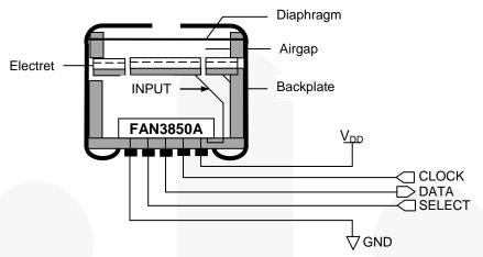
Figure 10. MIC Element Drawing
